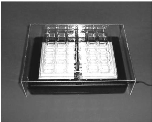
Transfer 20 (actively swimming) neonates with a micropipette into each rinsing cup in the sequence : row X (control), row 1 to row 5 (increasing concentrations of toxicant).
