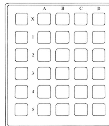
Each well of the test plates has to be filled with **5 ml** toxicant solution (or Standard Freshwater in the control column).
