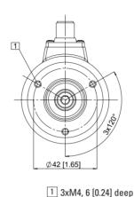
ø 58 mm, M12, M23 connector, cable versions Flange type 1 and 3 (Drawing with M23 connector)
